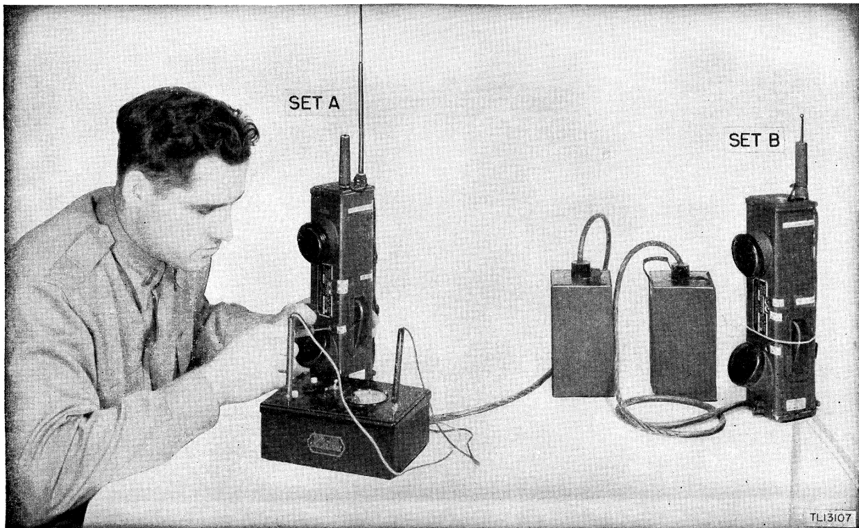
Figure 84. Emergency test equipment, using milliammeter.
